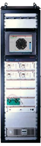
The RT-1000 Multichannel radio direction finder is designed for ATC (Air Traffic Control) and for VTS (Vessel Traffic Service). It is a very cost effective solution for applications where more than two simultaneous DF channels are required.
