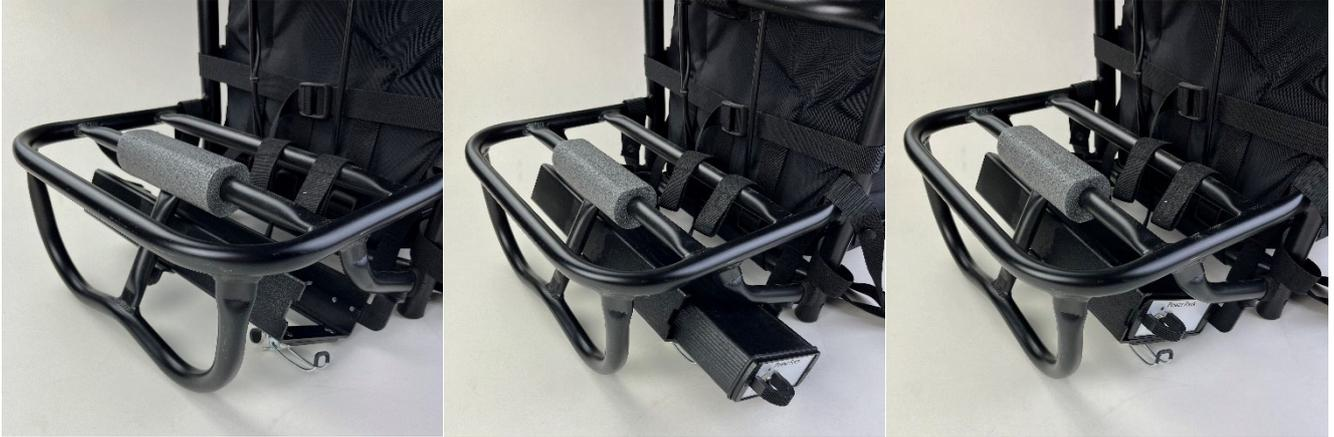
The power pack must be plugged into its rack as shown in the pictures above. As soon as the power pack is fully inserted, it must be fixed with the tension lock. This is located on the underside of the holder. When fixing the power pack, it is automatically connected to the backward connector on the carrying frame and ready for use.
