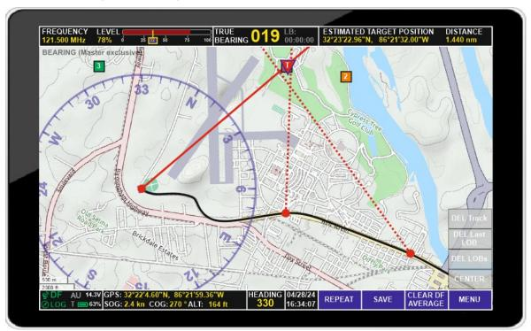
On the map display, the user's position is in the center of an azimuth dial (bearing rose), whose upper edge points toward the direction of the heading.
