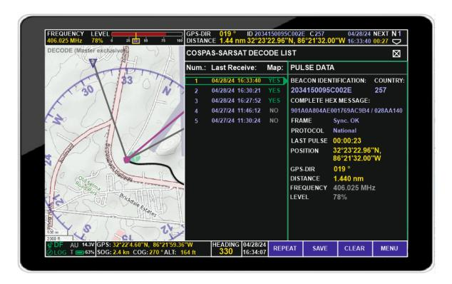
It consists of a list of received COSPAS-SARSAT messages, of which one can be selected, and the data decoded from the selected message.
