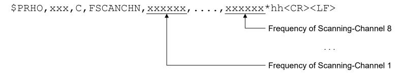
The answer to a successful FSCANCHN command will be the FSCANCHN data out sentence, which is described in chapter 5.2.15. If the operation was not successful, the answer is one of the three error sentences ERRCMD (5.2.24), ERRFIELD (5.2.25) or ERRRANGE (5.2.26).
