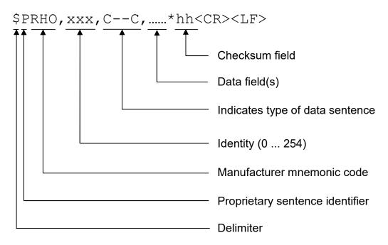
xxx is an identity field of numeric characters. The value is in the range of 0 to 254. The used format is without leading zeros. All data out from the DF is marked with the identity selected in setup. So the identity allows to separate data from different DF's connected to one RX.
