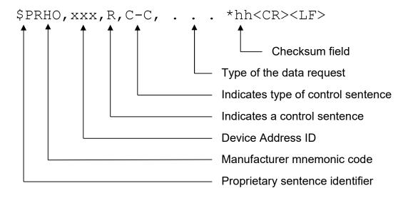
The DF only reacts to the request sentences if the Address ID in the sentence is 255 or is equal to the one set in the DF Setup/Interface/NMEA DF Remote/Remote Address ID. The address allows to access different DFs that are connected to one TX. C—C is a variable text field, which describes the type of data in this sentence.
