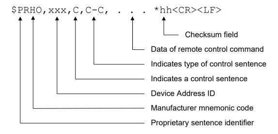
The DF only reacts to the control sentences if the address ID in the sentence is 255 or is equal to the one selected in the Setup/Interface/NMEA DF Remote/Remote Address ID. The address allows to access different DFs that are connected to one TX. c—c is a variable text field, which describes the type of data in this sentence.
