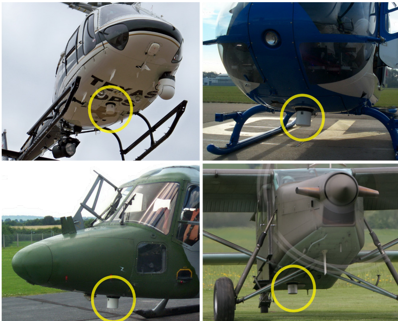
Fig 45) Antenna installed in good locations
