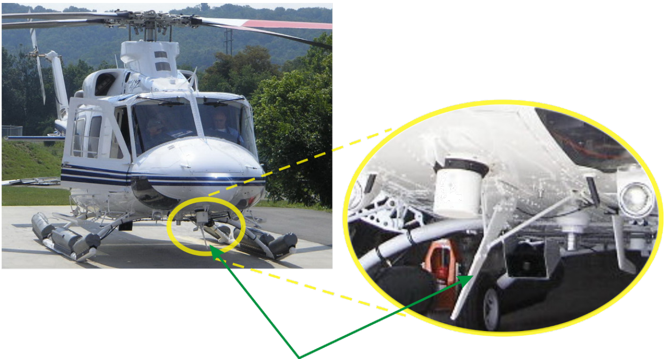
Fig 44) Antenna installed in a bad location
